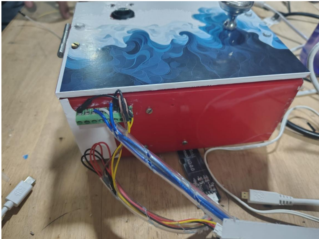
Fig 8.9 Cable sleeving of wires
