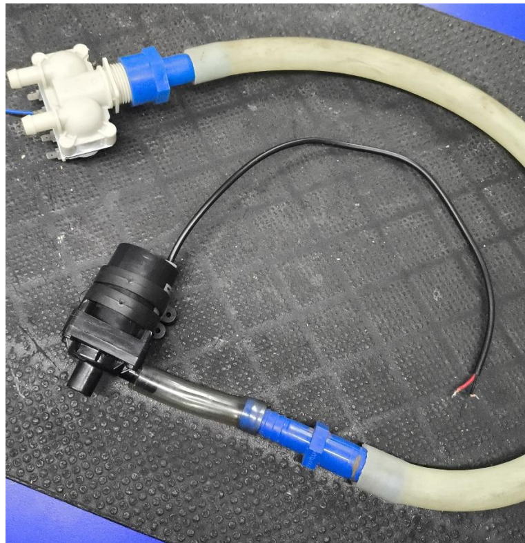
Fig 8.1 Pump–Solenoid Valve Connection Setup
